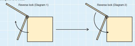
When a lid is being lifted, as shown in Diagram 1, a lock torque is applied in the closing direction, and the lid can be locked in at any position.
