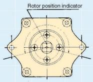
(Rotates ±105° with respect to the rotor position indicator)
