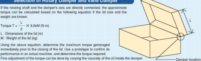
2) If the damper's rotating shaft and the lid's rotating shaft are connected by a lever or a gear, the results of the aforementioned torque calculation will vary according to the lever ratio or gear ratio.
