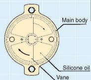
This is a rotating-type damper that utilizes the oil pressure. The braking force generated by oil viscosity, clearance between the rotor and the main body, and the vane's pressure-receiving area varies based on the structure shown above.
