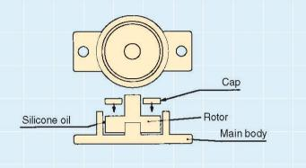
This is a rotary damper that utilizes the braking force generated by the oil's viscosity resistence. The braking force generated by oil viscosity, clearance between the rotor and the main body, and the oil's contact area varies based on the structure shown above.
